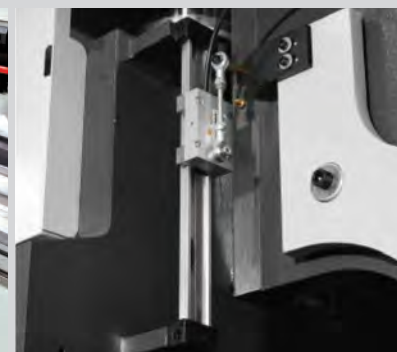
Bending compensation linear scales. Made in Italy
